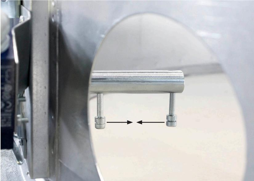
2. Press the pins together and insert the other end of the fuse to the other pin.
