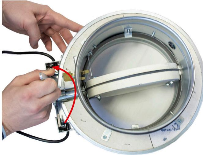
5. Push the fuse back in, keeping the blade in the open position. The shorter tooth of the fuse locks the blade in place.
